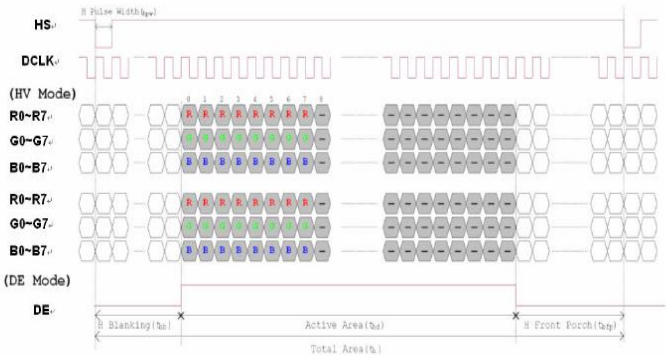
Figure 3. 1 Horizontal input timing diagram.
